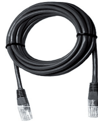
Ethernet Cable ** (thicker cable with RJ45 Connectors at each end)
